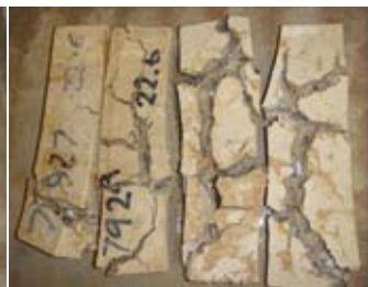
Plate 2 Failure of S3C (w/c 0.65) prisms after 570 days in 5% \text{Na}_2\text{SO}_4 at pH 3.5
