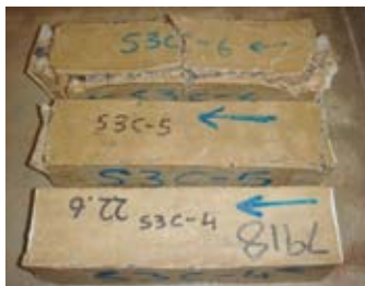
Plate 1 Failure of S3C (w/c 0.65) prisms after 570 days in 5% \text{Na}_2\text{SO}_4 at pH 7
